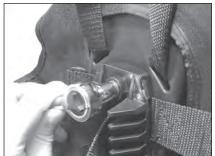
Step 8. Attach the Twin Cylinders
