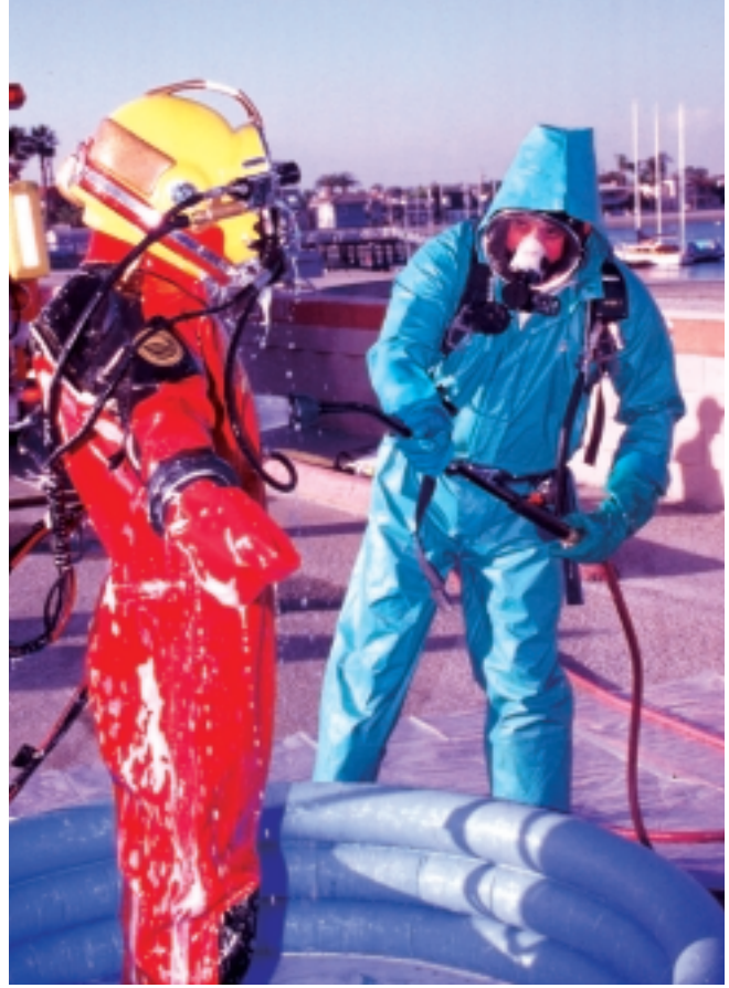
Photo #3: Decontaminating vulcanized rubber dry suits is relatively easy, compared to suits with a nylon exterior. (© Steven M. Barsky. All rights reserved.)
