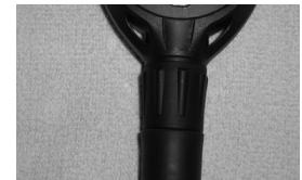
Fig. 118 - HPQD PROPERLY CONNECTED
