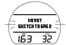
Fig. 68 - GAS SWITCH ALARM
