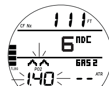
Fig. 60 - PO2 ALARM (during Audible)
