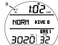
Fig. 3 - LOW BATTERY WARNING
